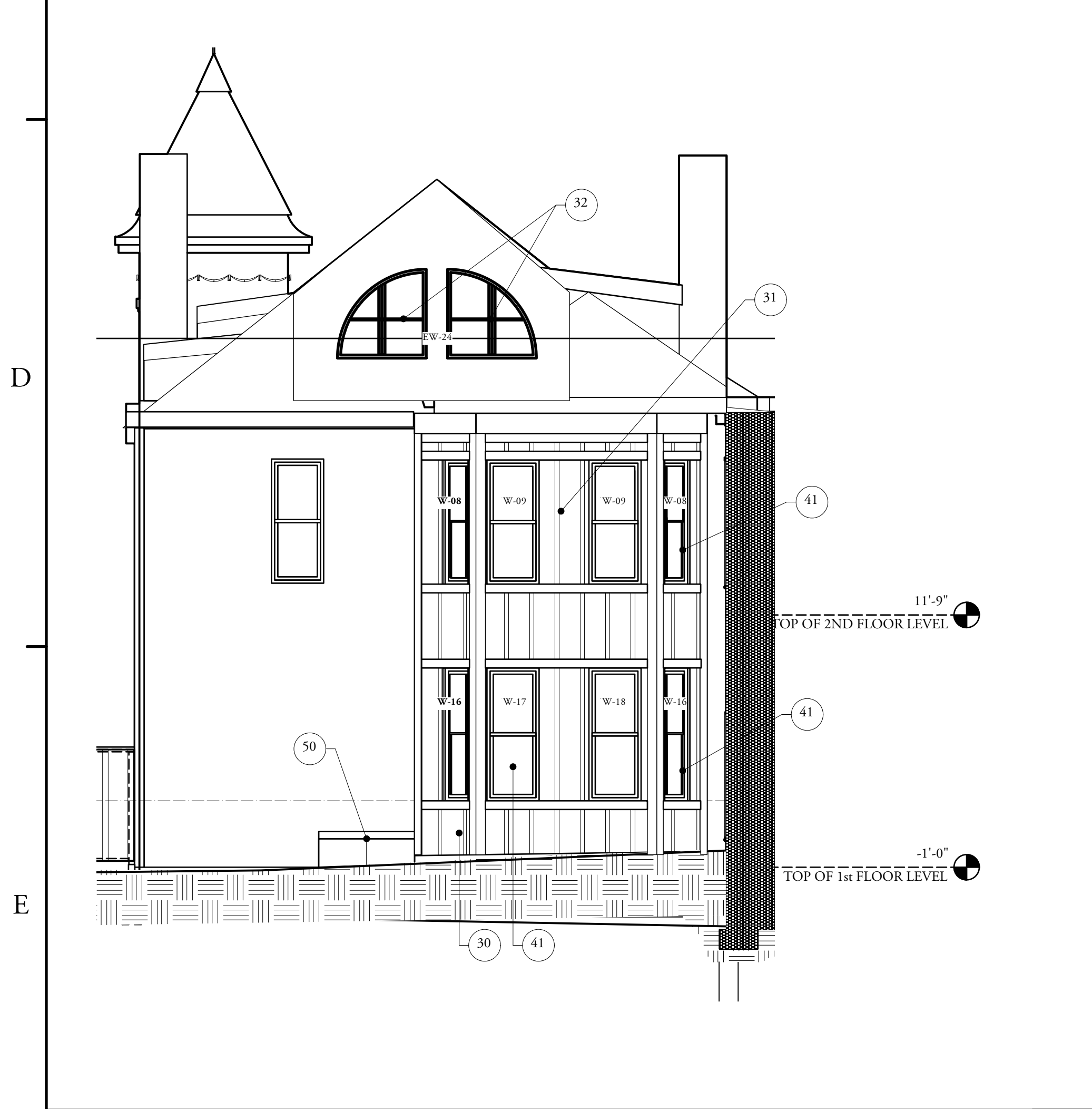
North Building Elevation/Section Scale: 3/16" = 1'-0"
